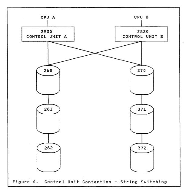
A head of string can be switched to either Control Unit A or Control Unit B but not both at the same time. A 'head of string' is busy when it or any of the devices on its string are transferring data. For example if data were being transferred from device 262 to Control Unit A and Control Unit B tried to access 261, a device busy condition would be returned to Control Unit B.
