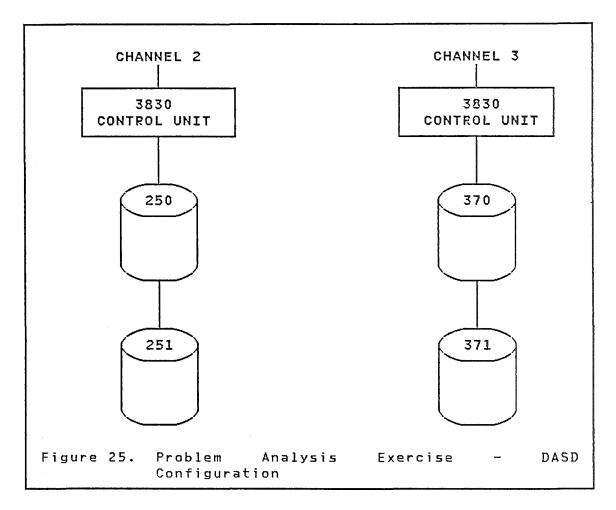
With only one channel path to a control unit, control unit busy conditions should not occur at the level shown for control unit 25X. However, further investigations of the configuration and the applications running when the data was collected, showed that:
